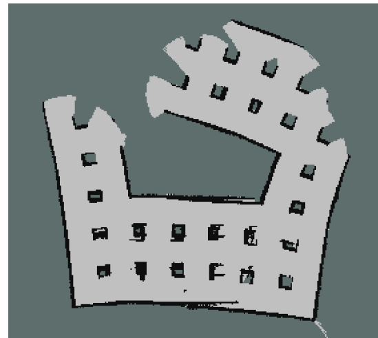
Fig. 8: Quality of the generate map fusion obtained from the two robots with an equilibrium strategy for a 9 minutes exposure time.
