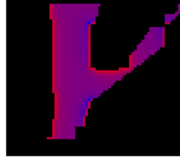
Fig. 4: (Left) is the potential field heat map generated by the created local planner with enhanced information from M . (Right) is the Configuration Space generated from M_T . It is interesting to note that the Configuration Space has blue pixels that represent frontiers.
